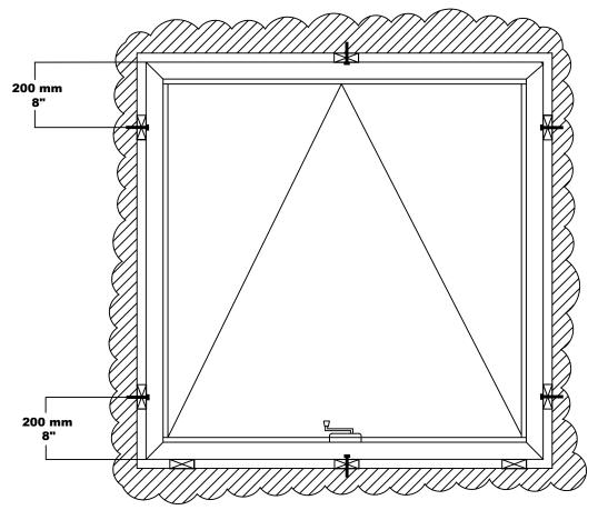
FASTENER LONG ENOUGH TO PENETRATE A MINIMUM OF 25MM (I") INTO THE ROUGH OPENING STUDS.
